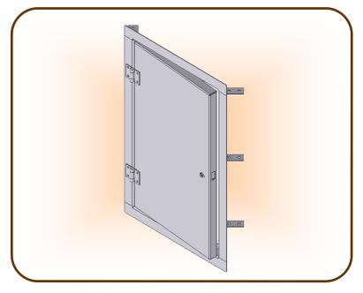
JCP Specifications: Access panel frames are fabricated from 7 gauge HRPO steel and the doors are fabricated from 10 gauge HRPO steel. The frame has a depth of 2-3/8" and flanges of 2-1/2". There will be a 1/8" clearance between the door and frame. The door is 2" thick with flanges bent around to the back on all sides for rigidity. The door will be flush with the face of the frame.
