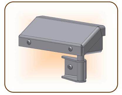
JCP Specifications: The JCP surface mount door position switch consists of a 12 gauge HRPO housing and mounting bracket, with a 1/2" diameter solid bar actuator shaft. Overall size of the housing is 6-1/4" long, 2-7/32" deep, and 1-27/32" tall. The housing and mounting bracket is secured with Torx® w/pin security screws.
